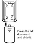
2 Slide 2 batteries into the compartment.
